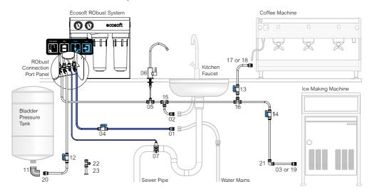
Some of the fittings shown on the diagram come from RObust package. These fittings can be used interchangeably or together with the fittings from RObust connection fitting pack when it's necessary to connect more than one appliance with %" or ½" female thread ports or a ¾" pressure tank. If any of your appliances have different thread sizes, use a suitable adapter for connecting it.
